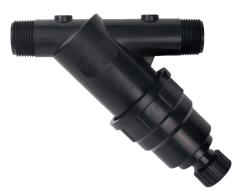
Plastic Spin Clean® Filters are unique screen filters that stay clean during operation. They effectively keep debris moving across the screen element towards the basin, where it is collected and can be drained to atmosphere.
