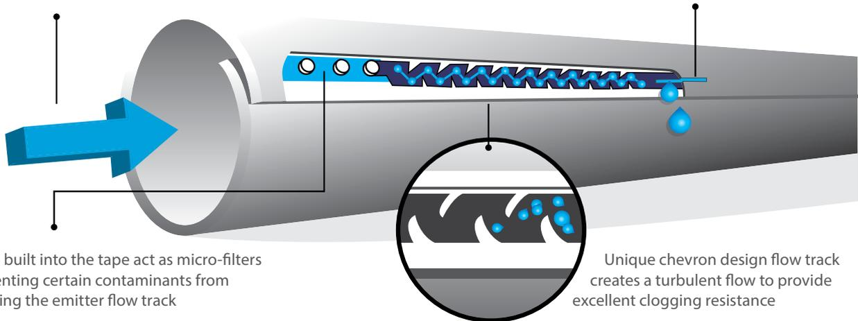
Inlets built into the tape act as micro-filters preventing certain contaminants from entering the emitter flow track
