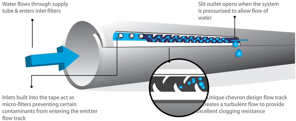
Most water will still contain foreign and organic particles even after it has been filtered. Therefore the design of the emitter is critical to help prevent clogging by stopping contaminants from entering the emitter.
