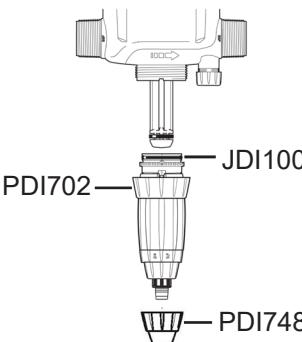
Cut 1" from the tip of the hose in a straight line. Insert the hose back onto the bottom of the check valve barb. Screw hose nut (PDI748) back on.
