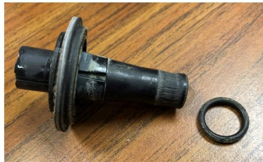
**Figure 8. Scarred throttling stem from a worn pressure regulator.**
