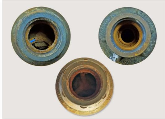
**Figure 7. Inlet and outlet of worn pressure regulators.**
