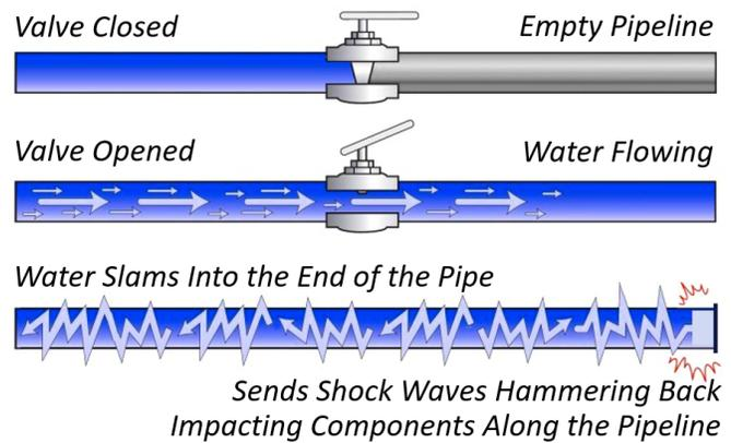
**Figure 9. (Water hammer, 2018) illustration of what happens inside pipes including water hammer**
