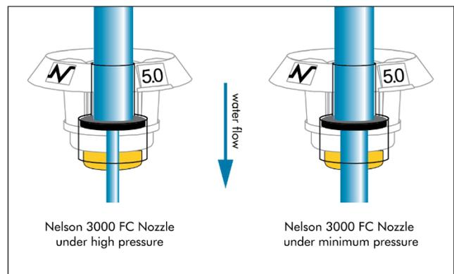
**Figure 11. Comparing outlet flow under high and minimum pressure.**
