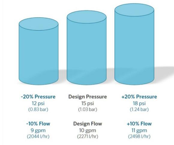
**Figure 1. A system is designed to operate at 15 psi (1.03 bar). If this same system experiences a 20% pressure variation, that will result in a 10% flow variation. That small flow variation can negatively impact sprinkler performance and affect your yields.**
