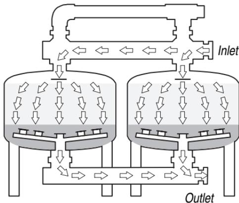
Sand media filters are effective at filtering both organic and inorganic contaminants. The large size and three-dimensional nature of a media bed provides more surface area and has greater holding capacity than many other types of filters. **Determining filter capacity and understanding the backwash function (cleaning) of your system are among the most important aspects of successful filtration.** These operations and more will be covered in the following pages.
